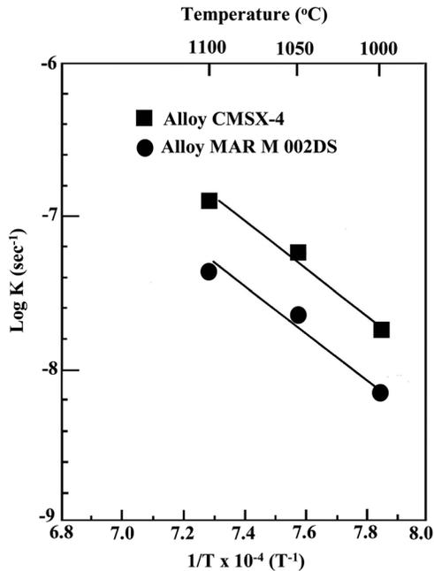
Fig. 7 Temperature dependence of the parabolic rate constant ( $K$ ) of interdiffusion between the bond coat and the superalloy substrates
