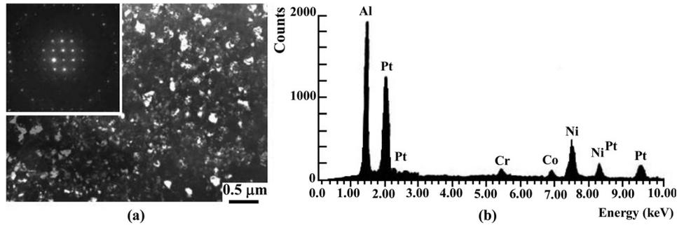
**Fig. 2** An example derived from the bond coat on alloy CMSX-4 illustrating the microstructure of PtAl<sub>2</sub> in the outermost coating layer in the as-deposited condition. (a) Dark-field TEM image formed with the [200] reflection; the inset is a microdiffraction pattern in <001> orientation consistent with the structure of PtAl<sub>2</sub>. (b) Corresponding energy dispersive X-spectrum illustrating the elemental composition of PtAl<sub>2</sub>.
