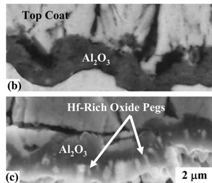
Fig. 8 Comparative oxidation behavior of the bond coat during thermal exposure at 1150 °C. (a) Thickening rate of the thermally grown oxide. (b) and (c) are backscattered SEM composition image showing the microstructures of the thermally grown oxide corresponding to alloys CMSX-4 and MAR M 002DS, respectively, after 48 h of exposure.
