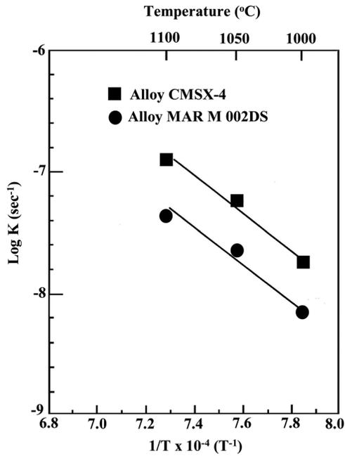
Fig. 7 Temperature dependence of the parabolic rate constant ( $K$ ) of interdiffusion between the bond coat and the superalloy substrates
