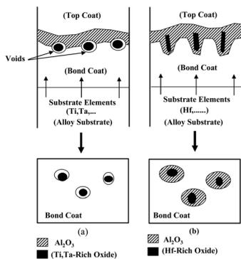
**Fig. 10** Schematics illustrating possible mechanisms leading to decohesion between the thermally grown oxide and underlying bond coat. (a) Alloy CMSX-4: coalescence of voids formed around Ta,Ti-rich oxide particles near the oxide-bond coat interface. (b) Alloy MAR M 002DS: fracture of Hf-rich oxide pegs.
