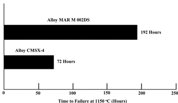
**Fig. 5** Comparative performance of the coating system on alloys CMSX-4 and MAR M 002DS as determined from thermal exposure tests at 1150 °C in air with a 24-h cycling period to room temperature
