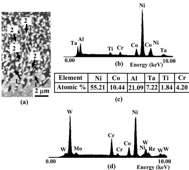
**Fig. 3** Analysis of the composition of interdiffusion zone of the coating on alloy CMSX-4 in the as-deposited condition. (a) Backscattered SEM composition image showing the microstructure of the interdiffusion zone. (b) Energy dispersive X-spectrum showing the elemental composition of the matrix phase (regions marked 1). (c) Composition of the matrix phase as determined by electron probe microanalysis. (d) Energy dispersive X-spectrum representative of the precipitates (regions marked 2).
